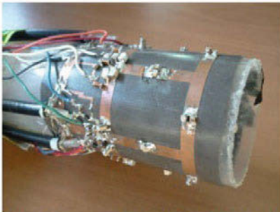
Fig. 1 Photograph of the four channel coil array built for rat head.
